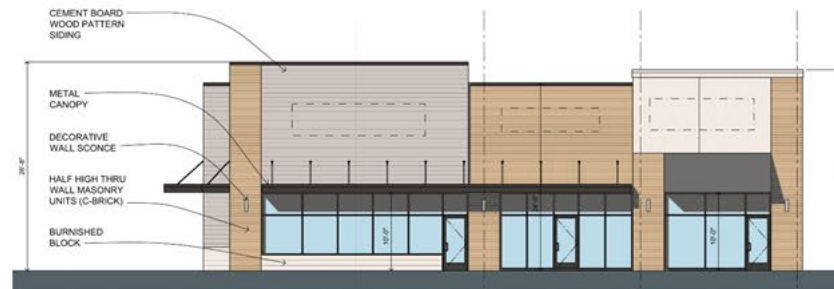
Bldg. A - South Elevation 1/8" = 1'-0"
