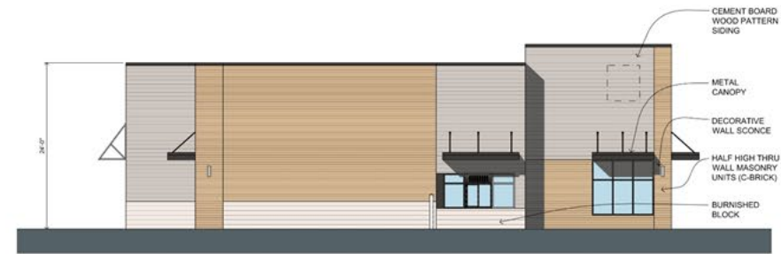
Bldg. A - West Elevation 1/8" = 1'-0"
