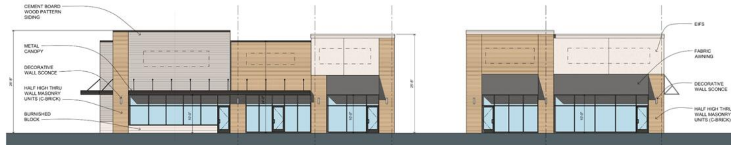
Bldg. A - South Elevation 1/8" = 1'-0"
