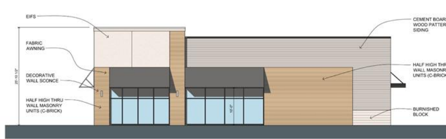
Bldg. B - East Elevation 1/8" = 1'-0"
