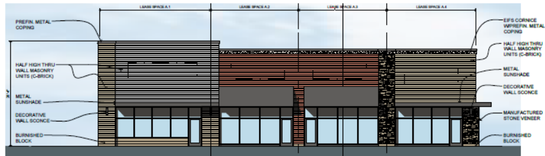
Bldg. A - South Elevation 1/8" = 1'-0"
