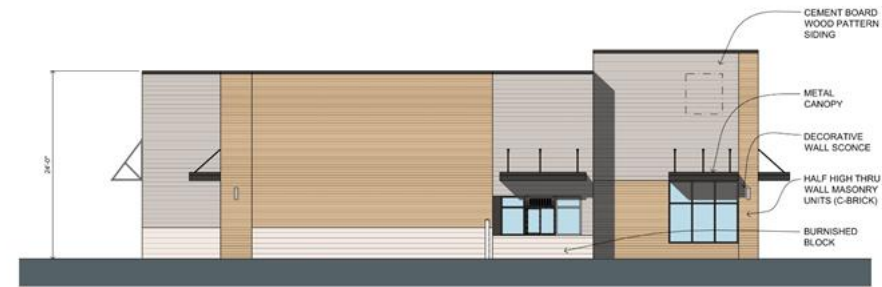
Bldg. A - West Elevation 1/8" = 1'-0"
