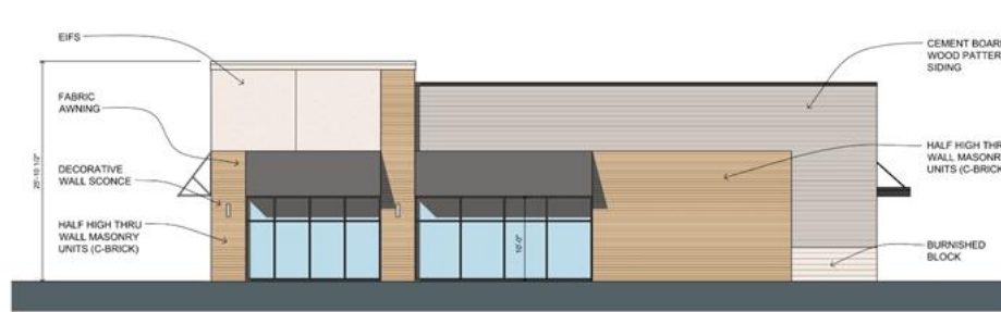
Bldg. B - East Elevation 1/8" = 1'-0"
